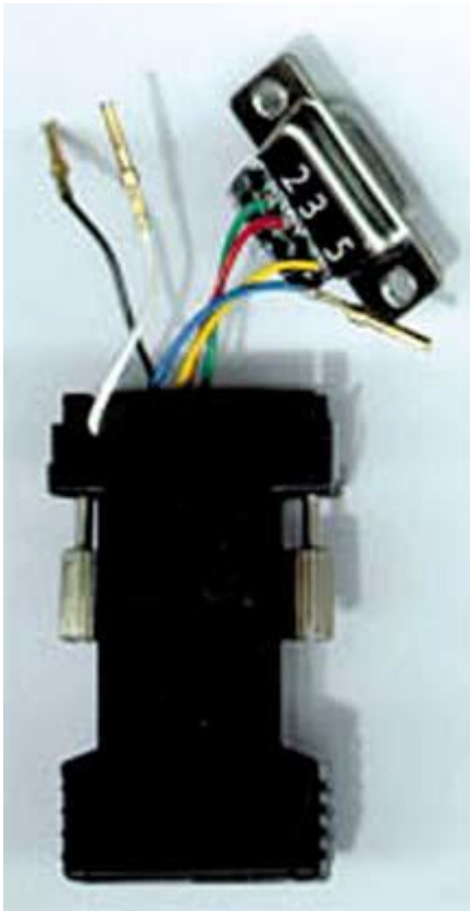
Figure 3. RJ12 to DB9 Wiring
